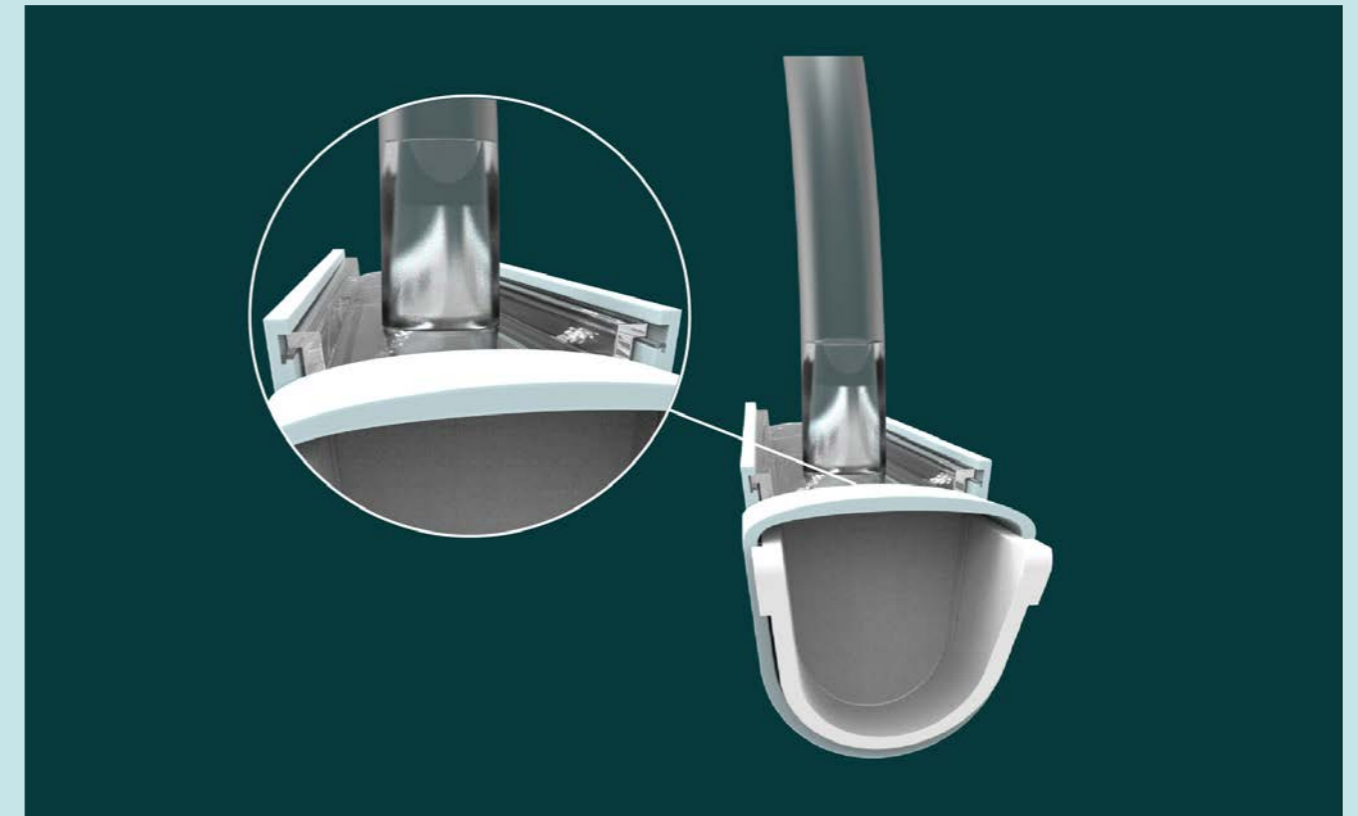
Figure 7.1.14: click mechanism of the window.
