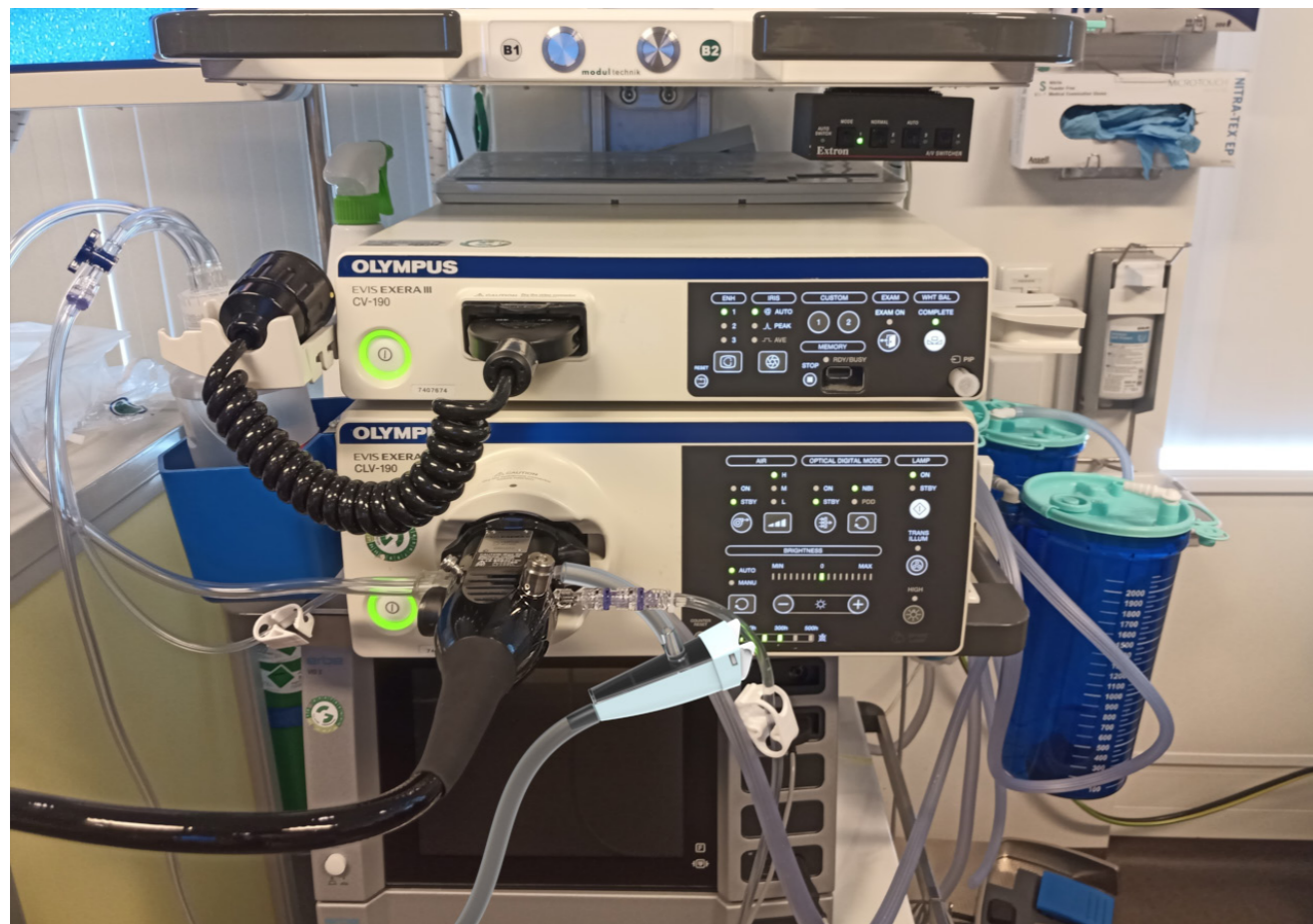
Figure 7.1.4: Rethink concept connected to endoscope.
