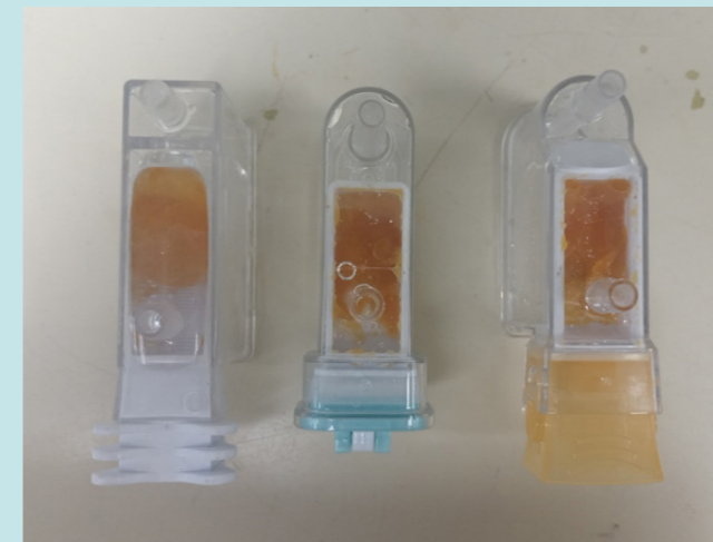
Figure 6.2.1: Polyp traps with 'clogged' drawers.
