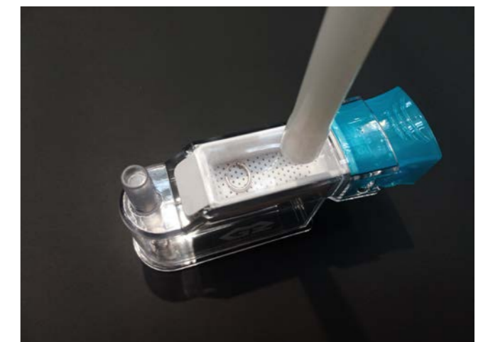
Figure 4.2.11: Magnifying window on the Endo-Safier
