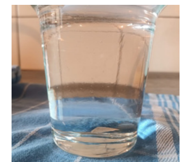
Figure E.5: Side view of float test results; PVC sample at bottom of glycerine filled glass.
