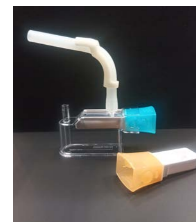
Figure 4.2.5: The Endo-Safier polyp trap with two drawers
